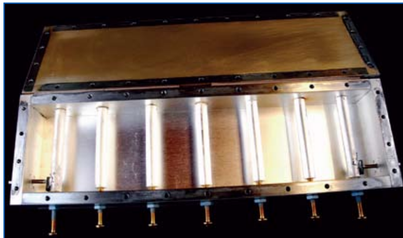
Figure 4: Inside a cavity filter
