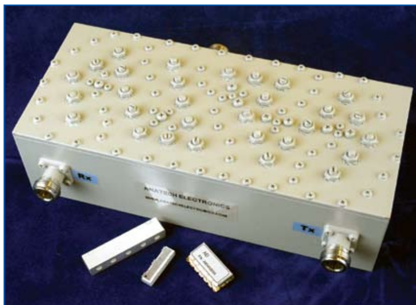
Figure 5: Size comparison between cavity and ceramic filters
