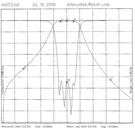
Marker 1 Freq 60.097MHz Atten -0.758dB Marker 2 Freq 20.162MHz Atten -42.614dB Marker 3 Freq 54.087MHz Atten -0.808dB Marker 4 Freq 66.107MHz Atten -0.902dB Marker 5 Freq 100.03MHz Atten -52.916dB Marker 1A Freq 59.903MHz Ret Loss -27.340dB
