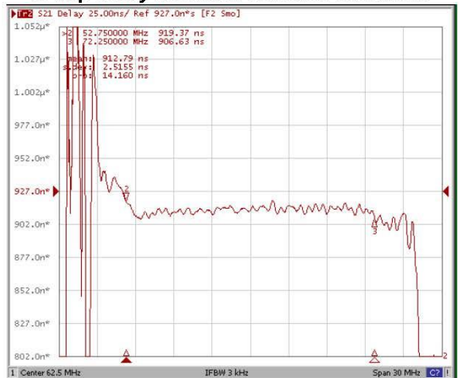
Group Delay Variation 62.5MHz \pm 9.75MHz
